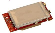
The module is equipped with a non-rechargeable battery.
